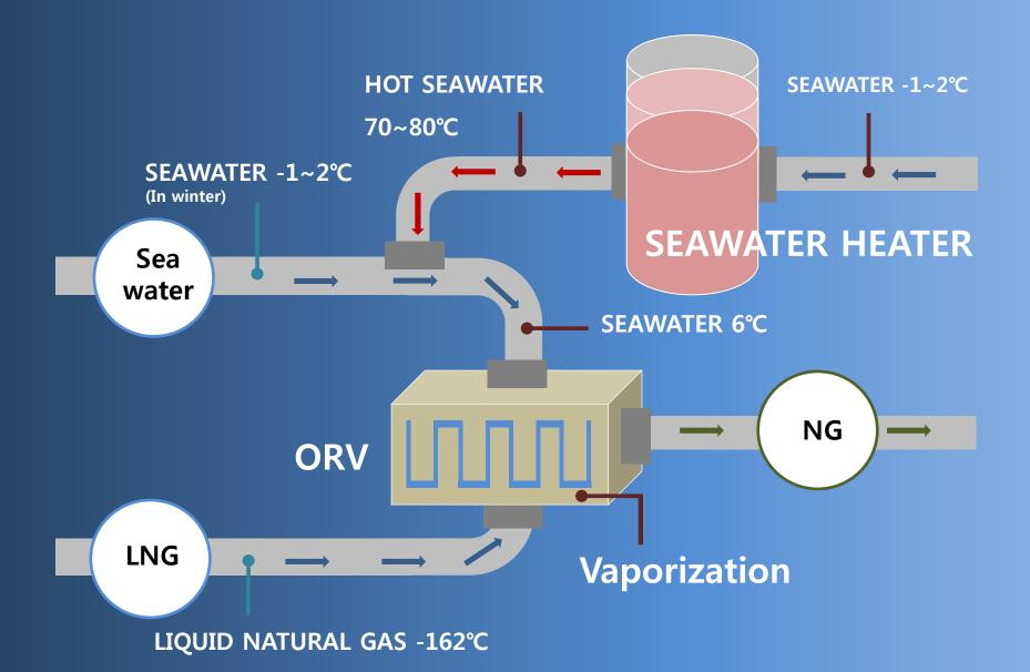
The SEAWATER HEATER of Kangwon NTS Co.,Ltd can supply 350~400 tons of seawater per time at the discharge temperature (set temperature). The seawater, heated by the SEAWATER HEATER, effectively improves the performance degradation of Open Rack Vaporizer (ORV) which is caused by the decrease in seawater temperature, thus maintaining the optimal temperature.
